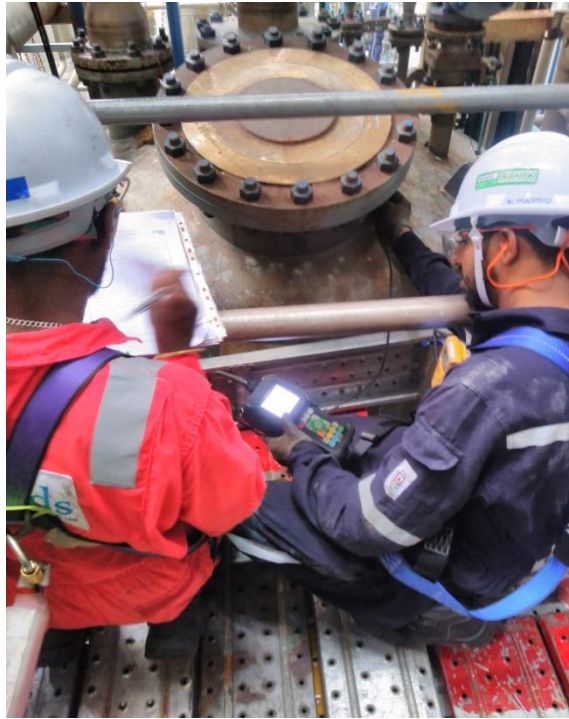
Photo 7: During Ultrasonic thickness measurement of nozzle head.
